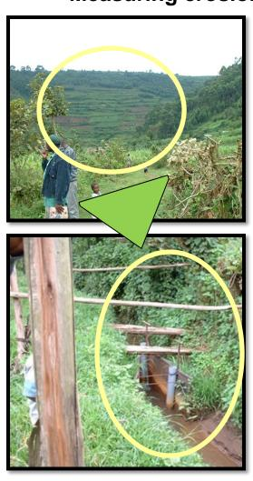
Topsoil loss from slopes upstream in the watershed (top) is assessed with a visual turbidity monitor (bottom).
